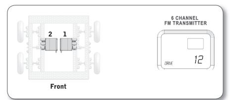
In this configuration, the first two control channels are mixed controls that affect both Motor Ports 1 and 2. The remaining joystick "control channels" controls their same-numbered motor ports directly.
