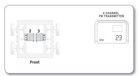
In this configuration, every joystick "control channel" controls its same-numbered motor port.
