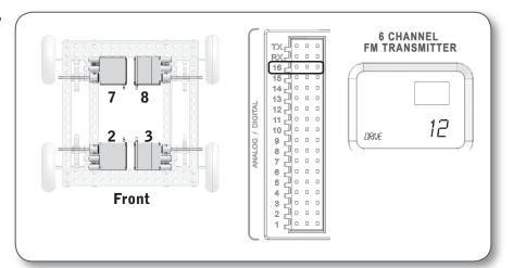
This configuration is the same as the basic "12 mode" as far as driving goes, except that the command mixes will drive both motors on the same side at once. Remember that the "Jumper 14" / "software 12 mix" mode will also allow the use of 4WD in an arcadestyle control, but with slightly different control characteristics (see original User Guide pages on control layout).
