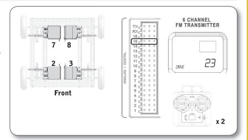
This configuration is the same as the basic dual-transmitter "23 mode" as far as driving goes, except that pushing the stick on the driver's transmitter causes both motors on the same side to be powered at once rather than just one.
