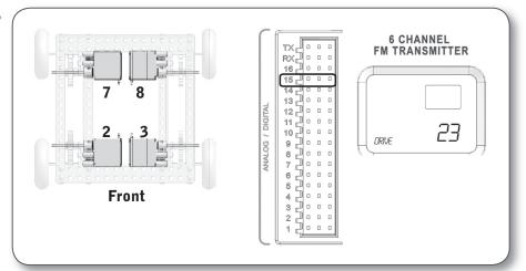
This configuration is the same as the basic "23 mode" as far as driving goes, except that pushing the stick causes both motors on the same side to be powered at once rather than just one.
