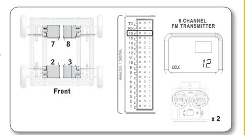
This configuration is the same as the basic dual-transmitter "12 mode" as far as driving goes, except that the command mixes from the driver's right-hand stick will drive both motors on the same side at once.
