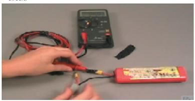
Place the BLACK wire of the multimeter in the end of the red wire which will be connected to the Vex controller, and wrap all exposed metal on it with electrical tape also. **Note:** it doesn't matter if the pins of the multimeter are switched. This will only make your readings negative.
