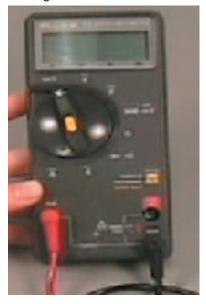
4. Set the multimeter's dial to the "A" which has two flat lines over it, one of them dotted. You have now set the multimeter to measure Direct Current.
