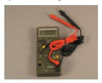
**3.** Use the multimeter to measure the voltage of the battery. Attach alligator clips to both the red and black leads. If your alligator clips are colored, always attach red to red and black to black. Attach the snap-on piece to the battery. Attach the red alligator clip to the red wire leading from the battery's anode (+) and attach the black alligator clip to the black wire leading from the battery's cathode (-). Record the Multimeter value in the appropriate place on your worksheet.
