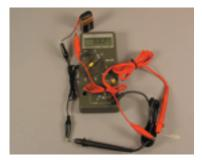
**4.** Prepare the multimeter to measure resistance. Plug the red lead into the voltage/resistance port, and the black lead into the com port. Switch the multimeter selector to Ohms (usually marked by the Greek letter Omega).
