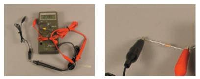
6. Prepare the multimeter to measure direct current amperage. Plug the red lead into the amperage port, which is usually marked with an A, and the black lead into the com port. Switch the multimeter selector to direct current amperage (on most multimeters, it is marked by an A with a straight line and a dotted line over it.)
