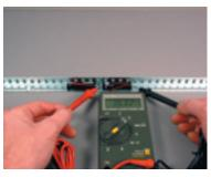
**9.** Measure the anode (+) to cathode (-) voltage of the third battery with the multimeter. Record the value on your worksheet beside " $V_{CD}$ ".
