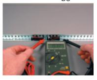
5. Place the two batteries in series on the long angle rail. The cathode of battery 1 should touch the anode of battery 2. Place the red lead on the cathode of battery 2, and the black lead on the anode of battery 1. Record the value on your worksheet beside "V<sub>CA</sub>".
