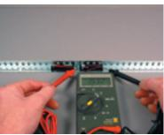
**9.** Measure the anode (+) to cathode (-) voltage of the third battery with the multimeter. Record the value on your worksheet beside "V<sub>CD</sub>".
