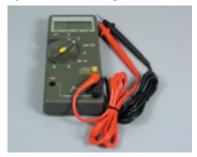
**3.** Place a battery on the long angle rail. Measure the anode (+) to cathode (-) voltage with the multimeter by placing the red lead on the anode, and the black lead on the cathode. Record the value on your worksheet beside "VAB".
