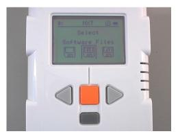
**Select "Software Files"** Press the orange button again to go into the "Software Files" menu.
