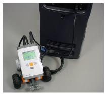
**3.** Place the robot on an open area on the floor or table. In the Program Debug window, press the button labeled "Start". The ROBOTC debug windows appear when the download is complete.
