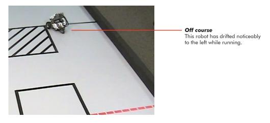
Even when you set the motors to go the same speed, the robot turns a little. Recall that a turn results from two motors moving at different speeds.
