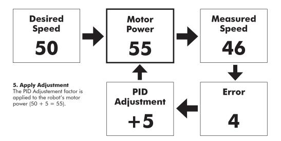
The new motor power is calculated by adding the PID adjustment factor to the original power.
