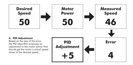
Based on the size of the error term, and how the error has been changing over time (has it been getting bigger or smaller?), the PID algorithm calculates an adjustment to the motor power that should help the motor's actual speed to get closer to the desired speed.
