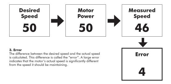
How far off is the speed? The "error" term is simply the difference between the measured speed and the desired speed.
