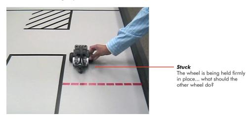
Using PID, the other motor will keep running at the speed it was set to, and the robot will begin to spin in a circle as if ordered to turn.
