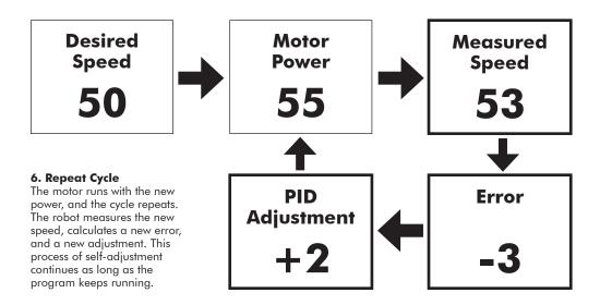
The adjustment is applied to the motor power. The speed is measured again. The error is recalculated (hopefully it is now smaller!). A new adjustment factor is determined. The cycle continues forever, always ready to catch and compensate for any factor that may make the robot go at the wrong speed.
