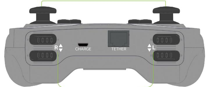
These buttons turn the motors on at full speed in one direction.
