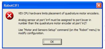
**Note:** The Potentiometer can be plugged into any of the Analog / Digital ports (in1 through in16). Any digital sensors (Limit Switches, Bumper Switches, Encoders, Ultrasonic Rangefinders) must be used in higher Port numbers for them to be configured correctly.
