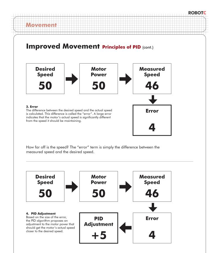
Based on the size of the error term, and how the error has been changing over time (has it been getting bigger or smaller?), the PID algorithm calculates an adjustment to the motor power that should help the motor's actual speed to get closer to the desired speed.
