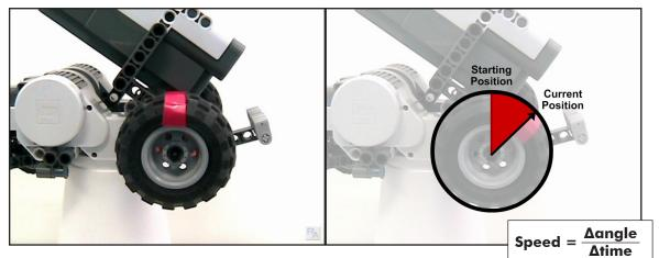
**Starting position (t=0)** The initial position of the wheel as it starts turning.
