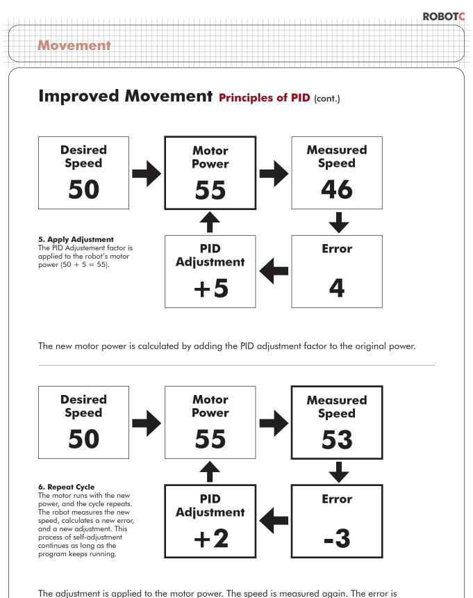
The adjustment is applied to the motor power. The speed is measured again. The error is recalculated (hopefully it is now smaller!). A new adjustment factor is determined. The cycle continues forever, always ready to catch and compensate for any factor that may make the robot go at the wrong speed.
