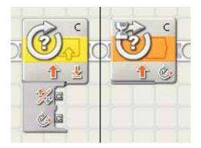
The block on the left is the yellow Rotation Sensor block, configured to reset the rotation sensor (as seen in the Continue section activity "There and Back (2)"). The block on the right is the orange Wait For block, configured to wait for the rotation sensor to reach a certain value in the forward direction, so we commonly call it the Wait For Rotation block.
