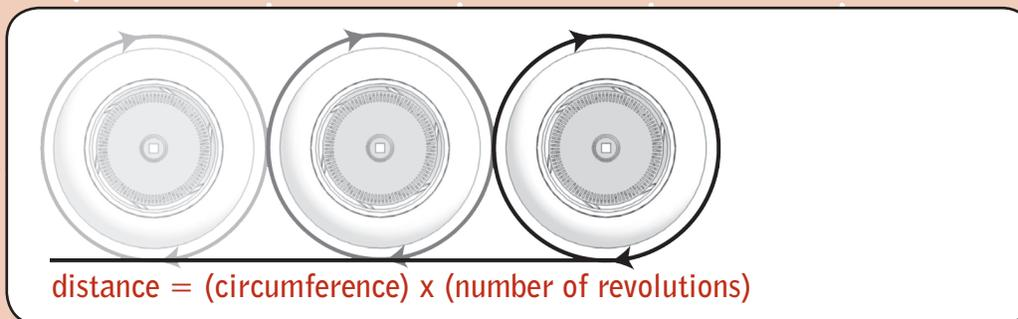
For a standard wheel in the Vex Inventor's kit, the diameter is 2.75". So the distance the wheel travelled would be:
