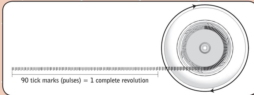
By mounting a shaft encoder on the axle of one of your robot's wheels, you'll be able to determine how many times that wheel has rotated. That, in turn, can be used to calculate the distance the robot has travelled, based on the diameter of the wheel.
